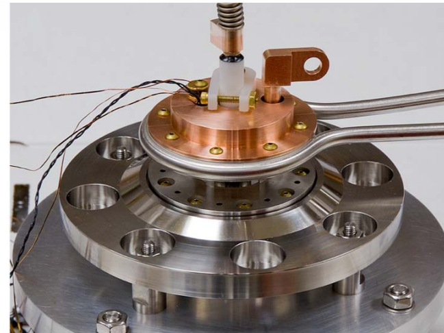
Cryogenic cooling of liner targets has been demonstrated (liquid D2)
